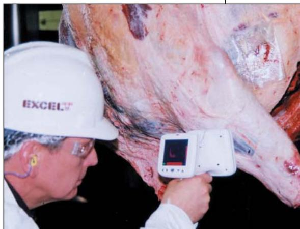
Emerging “pre-intervention” technologies, such as this prototype of a handheld scanner to detect fecal contamination being tested by Excel Corp., are being introduced with increasing frequency. (Photo courtesy of eMerge Interactive)
